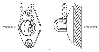
Hold the tension device and the bracket against the window frame or wall and then move it upward at least 1/4" - mark the position of the bracket (mark the location of the screw holes with a pencil).
